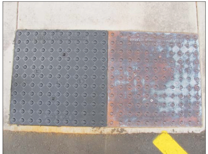
10/15/2012 Right side: wet coated of original CorrVerter. Left side: Dry CorrVerter Black
