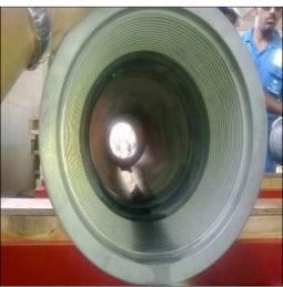
Using VpCI®-422, Weatherford's drilling tools were successfully cleaned and restored. The tools then received a spray coating of a 5% solution of Cortec's VpCI®-414 to provide additional corrosion protection for up to 3-4 weeks. This process has nearly eliminated the part rejection rate, reduced the cleaning period, and enabled huge cost savings compared with machining-based
