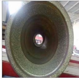
**Drilling Tools After Rust Removal using VpCI®**
